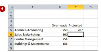
The macro enters a formula into the current cell. The formula calculates 15% more than the value one cell to the left and truncates that value to an integer. This final value is entered into the current cell.
