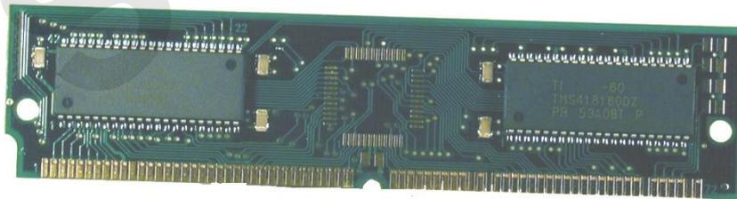
So RAM is volatile, meaning that its contents will be lost as soon as there is an interruption to power. RAM is also constantly changing with new contents flowing through on a regular basis.
